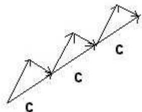
The bottom vector  $c$  is added three times which is equivalent to multiplying it by 3.
