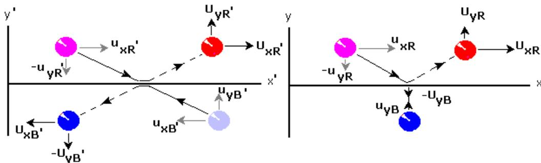
View of observer who is travelling at a velocity intermediate between that of the balls. (Red = +v Blue = -v Observer = 0 m/s)
