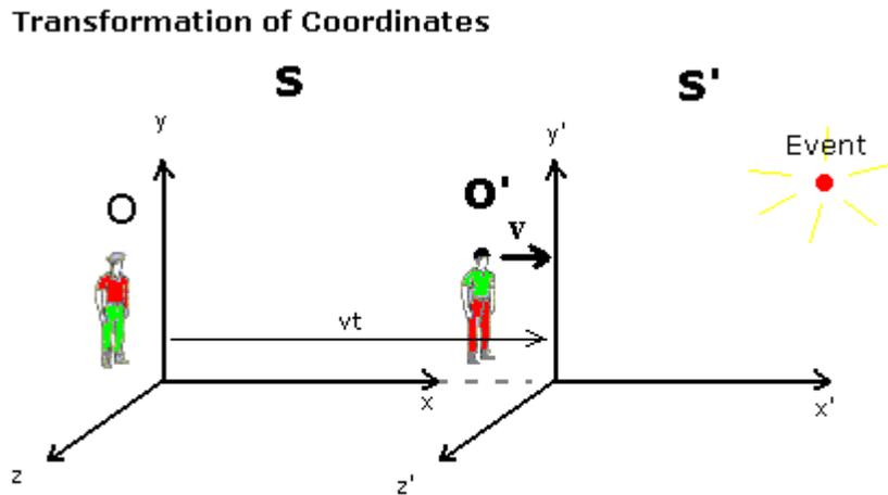
The observers are moving at a relative velocity of  $v$  and each observer has their own set of coordinates  $(x, y, z, t)$  and  $(x', y', z', t')$ . What coordinates do they assign to the event?
