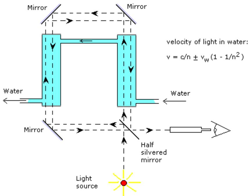
The special theory of relativity predicts the result of the Fizeau experiment from the velocity addition theorem without any need for an aether.
