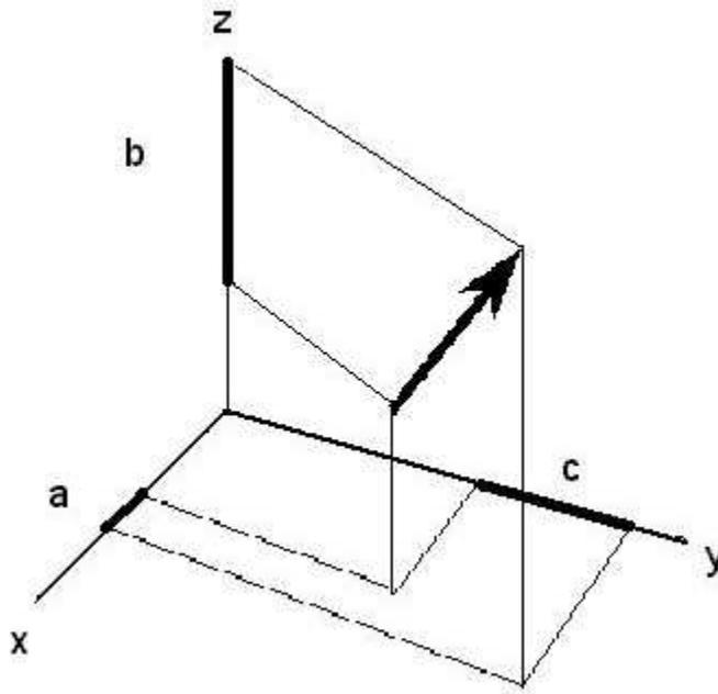
The vector represented by the bold arrow has components  $a$ ,  $b$  and  $c$  which are lengths on the coordinate axes. If the vector starts at the origin the components become simply the coordinates of the end point of the vector and the vector is known as the position vector of the end point.
